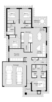
OVERALL WIDTH- 10.89m OVERALL LENGTH- 20.89m MIN BLOCK WIDTH- 12.5m MIN BLOCK LENGTH- 25m
