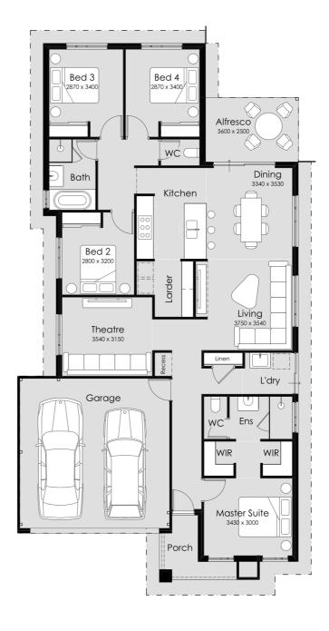
OVERALL WIDTH- 10.89m OVERALL LENGTH- 20.89m MIN BLOCK WIDTH- 12.5m MIN BLOCK LENGTH- 25m TOTAL AREA- 191.94m<sup>2</sup>
